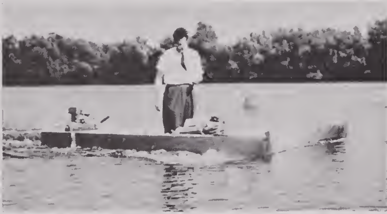
FIGURE 48. Equipped with outboard motor, M-29 Weasel floats in water and achieves speed of 1.5 mph.
